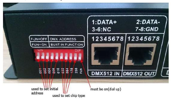
• Controllable chips: the sixth to ninth switches are used to set the chip type, H805DMX controls maximum 170 pixels.
