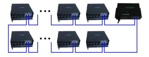
(3). The use of optical fiber, makes further transmission distance. You can connect port1 to slave controller with optical fiber. If you want to connect port2 to slave controller, connect slave controller to slave controller with optical fiber, an IP converter is needed.
