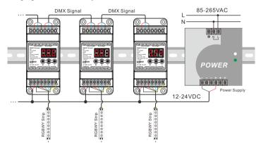
4CH Constant Voltage Decoder/RJ45 Input Voltage: DC12V-24V
