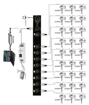
$Note: When using 818-RDM \ master to \ control \ several \ DMX \ slave \ devices, \ according \ to \ DMX512 \ protocol$ a small metal film resistor of 90~120 Ω1/4W should be welded at the end of each DMX signal line (between signal + and signal-).
