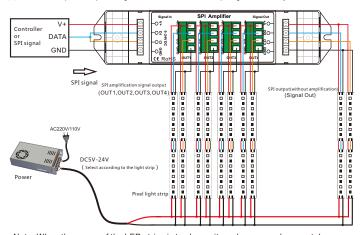
Note: When the power of the LED strips is too large, it can be powered separately. The LED strips are separately connected to the power supply, and the V+ of the amplifier is not connected.
